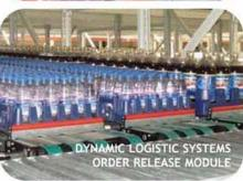
Colo., USA) presented its Order Release Module, a mechanized buffer and sorting module for fully automatic order picking of a variety of packaging types. It has been installed in a major US CSD bottler, picking at about 5,500 cases per hour. nedcondls.com • dematic.us • slg.com
